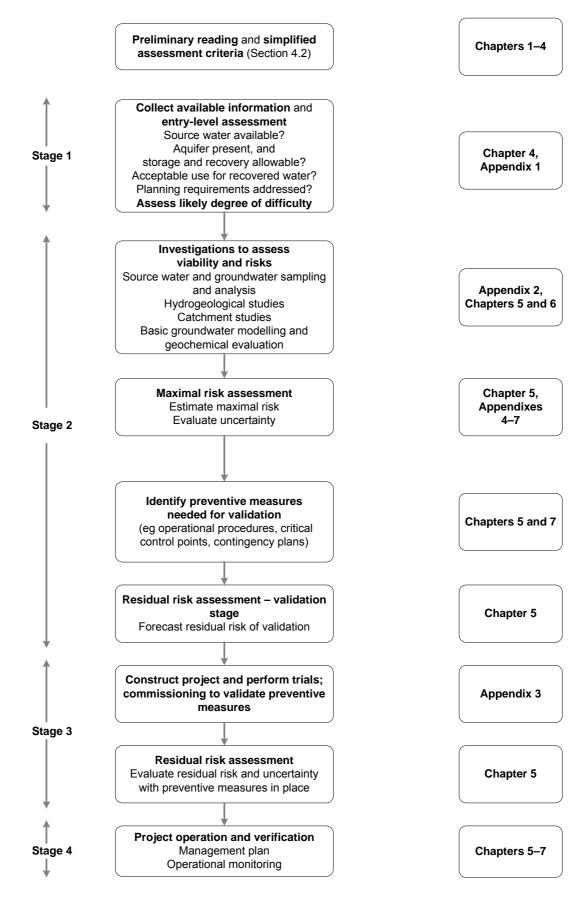
Figure 1.3 How to use the managed aquifer recharge guidelines to assess and manage risk
